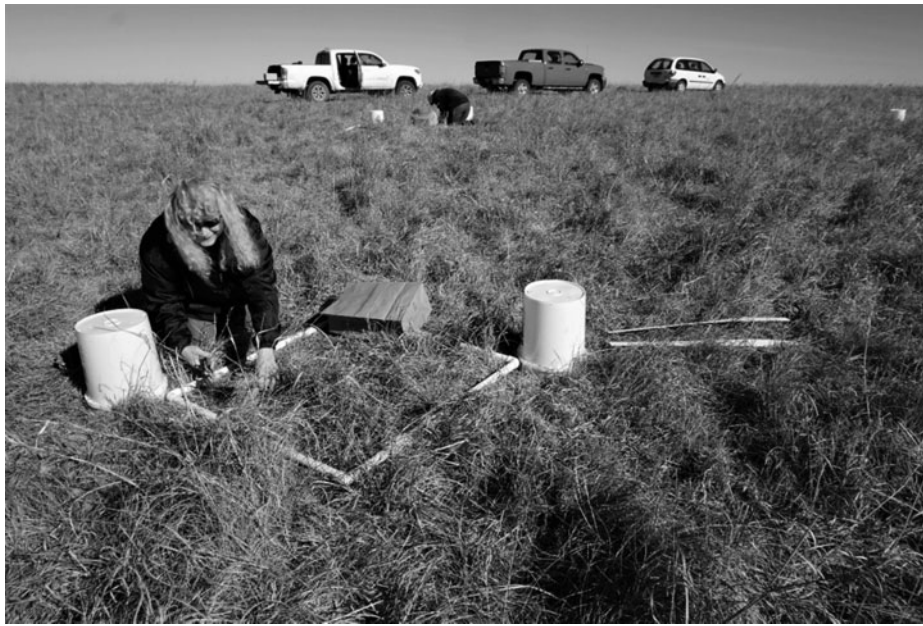
Fig. 1. Clipping of aboveground biomass within a 1 m 2 area outlined with white PVC piping. Two upturned buckets at opposite corners of the clipped area served as ground-level references and two parallel white vinyl strips served as location identifiers.
