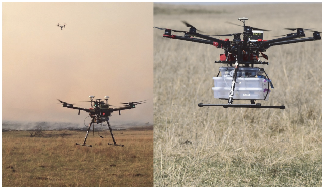
Figure 1. Photos of UAS 1 for continuous measurements (left) and UAS 2 for integrated sampling (right).
